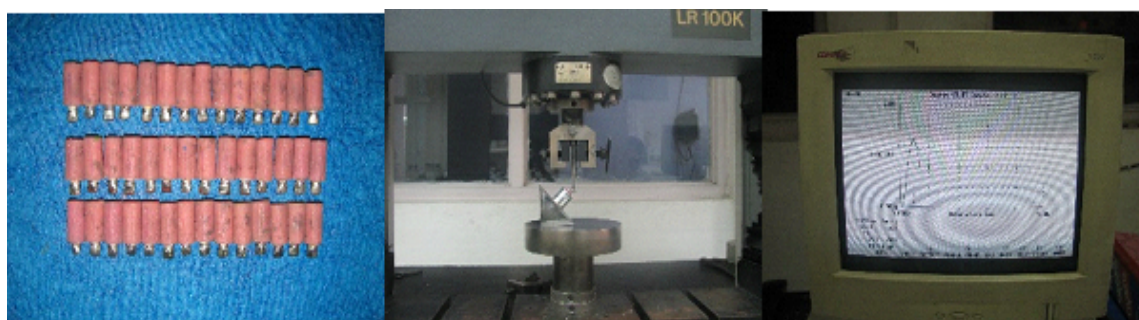
Figure 2: (a) Final samples ready for testing procedure, (b) Samples testing in UTM, (c) Stress strain graph
