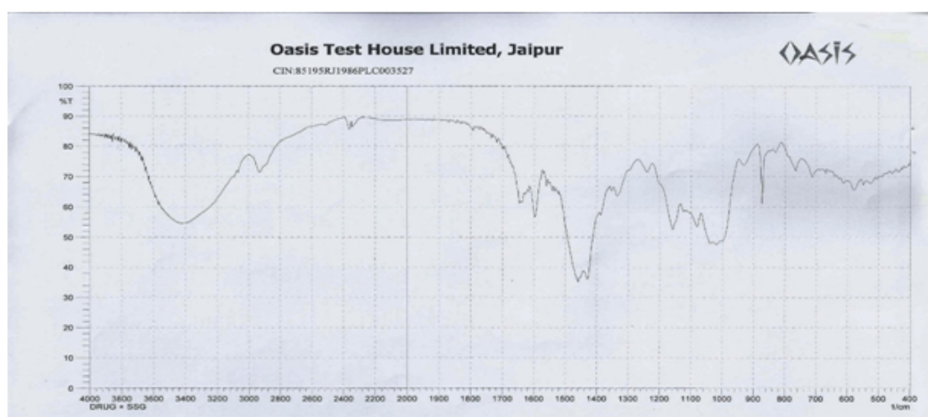
Figure 2: FTIR Spectrum of Lornoxicam + Sodium starch glycolate
