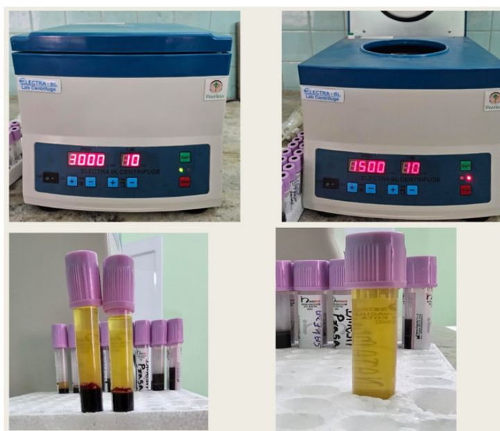
Figure 1: PRP prepared using A double-spin centrifuge protocol to concentrate platelets in which first the blood withdrawn was centrifuged at 3000 rpm for 10 minutes followed by a speed of 1500 rpm for same time.
