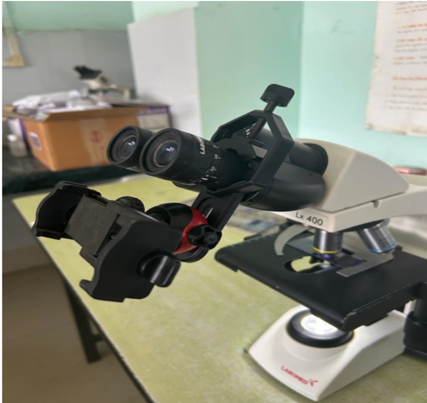
Figure 2: Sequential workflow of adapter mounting and live telepathology setup showing independent assembly of the modular unit, attachment to the microscope eyepiece, smartphone mounting with optical alignment, and the final ready-to-use live transmission setup.
