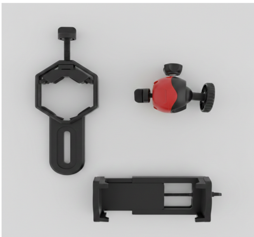
Figure 1: Compact modular smartphone microscope adapter fabricated from commercially available components showing the eyepiece clamp, adjustable alignment unit, ball-head mount, and smartphone holder compatible with routine laboratory microscopes.
