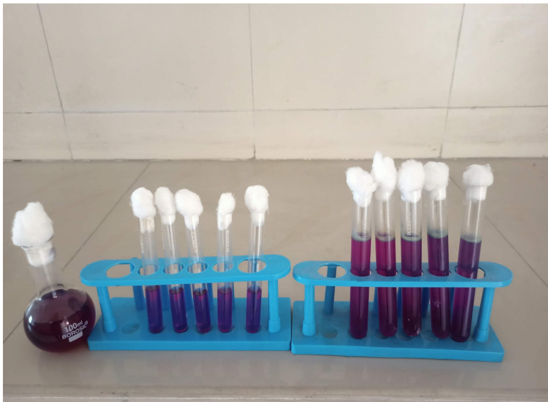
Figure 4: Presumptive coliform count performed using multiple tube method in the laboratory.
