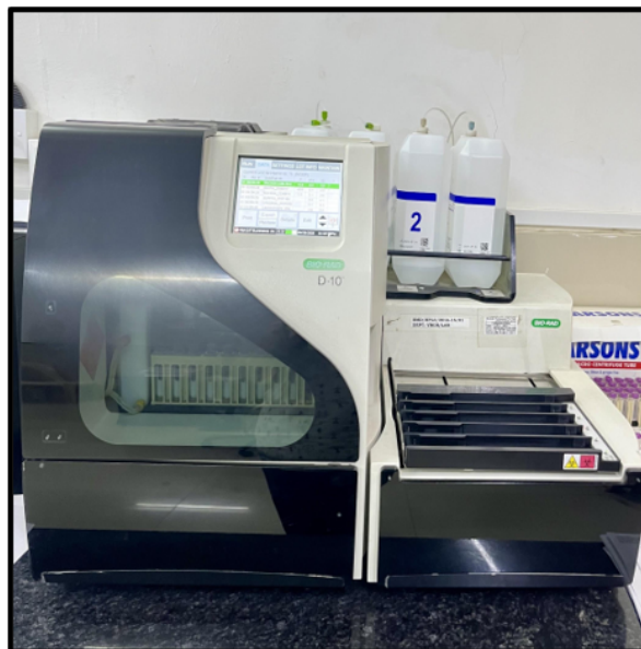
Figure 1: Bio RAD D-10 analyser for HPLC analysis [HPLC- High performance liquid chromatography]
