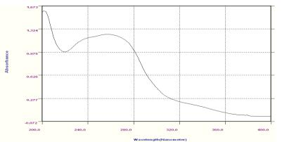
Figure 4: UV spectrum of Imatinib mesylate.
