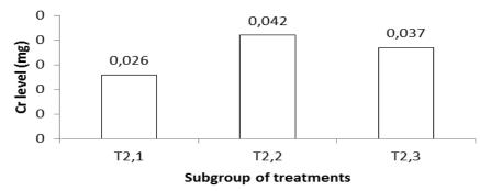
Figure 2: Comparison of the amount release of Cr from dental archwires between subgroup of treatments. T<sub>2,1</sub>: normal saline; T<sub>2,2</sub>: 1% lactic acid; and T<sub>2,3</sub>: normal saline + isotonic drinks.
