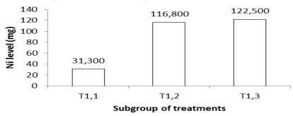
Figure 3: Comparison of the amount release of Ni from dental archwires between subgroup of treatments. T<sub>1,1</sub>: normal saline; T<sub>1,2</sub>: 1% lactic acid; and T<sub>1,3</sub>: normal saline + probiotic drinks.
