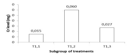
Figure 1: Comparison of the amount release of Cr from dental archwires between subgroup of treatments. T<sub>1,1</sub>: normal saline; T<sub>1,2</sub>: 1% lactic acid; and T<sub>1,3</sub>: normal saline + probiotic drinks.
