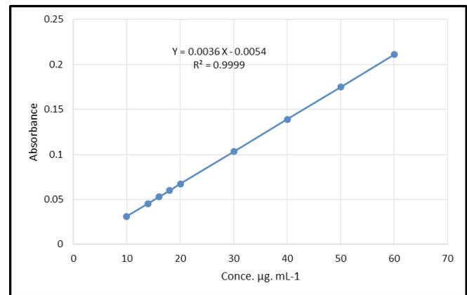
**Figure 6:** Calibration curve of the complex
