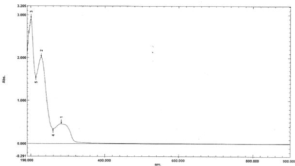
**Figure 3:** Spectrum of Indomethacin Absorbance (λ<sub>max</sub> 280.5 nm)
