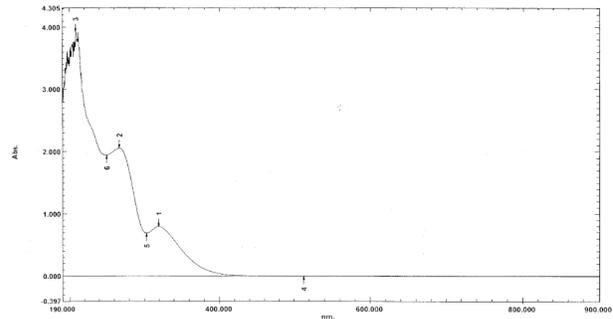
**Figure 5:** Absorbance spectrum of complex (λ<sub>max</sub> 319 nm)
