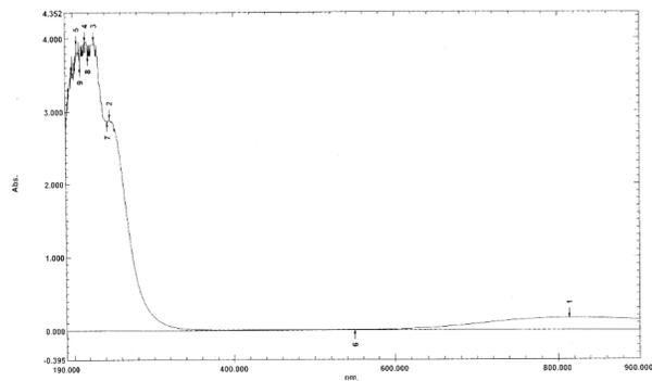
**Figure 4:** Absorbance spectrum of CuCl (λ<sub>max</sub> 814 nm)
