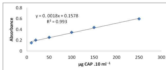
**Figure 3:** The effect of the oxidant amount
