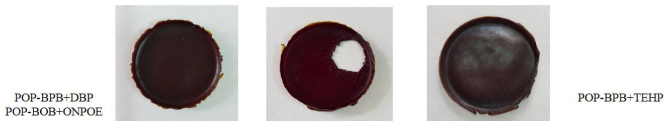
Figure 3: Manufactured membranes of POP using several plasticizers
