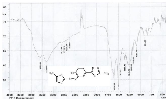
Figure 2: FTIR spectrum of compound (2)
