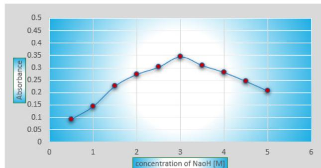
**Figure 4:** The impact of sodium hydroxide concentration on the color development in the determination of  $10 \mu\text{g/mL}$  ( $\text{LPZ}$ )
