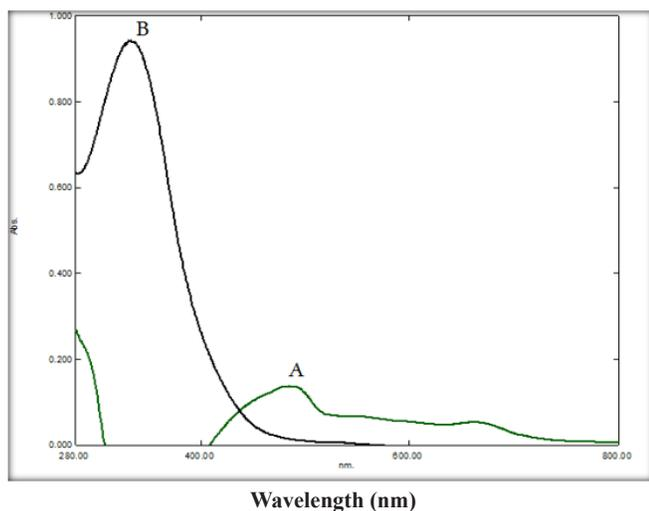
**Figure 1:** Absorption spectra of (a) 10 µg/mL LPZ versus reagent blank, (b) blank solution versus dissolvent under initial test conditions
