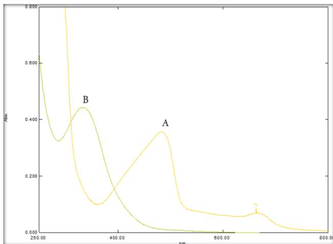
Figure 6: Absorption spectra of (a) 10  $\mu\text{g/mL}$  (LPZ) versus reagent blank, (b) blank solution versus solvent under the optimum conditions
