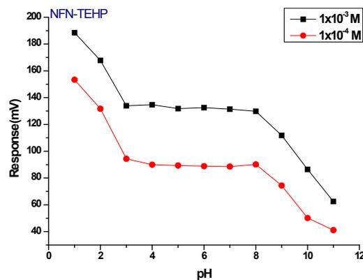
Figure 12: Effect of pH on NFN-TEHP electrode response
