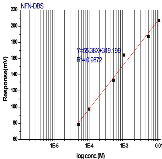
Figure 5: Calibration curve NFN-DBS.
