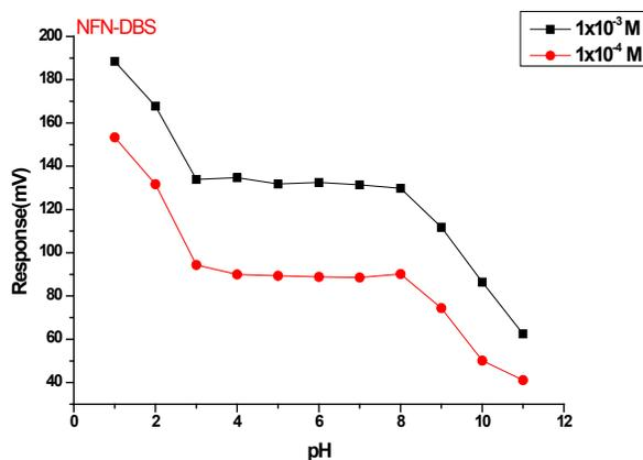
Figure 13: Effect of pH on NFN-DBS electrode response
