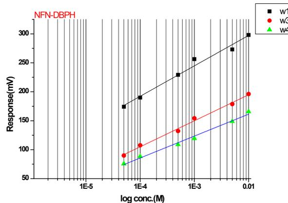
Figure 11: Lifetime of the (NFB-DBPH) electrode.
