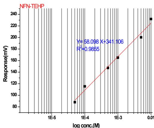
Figure 3: Calibration curve of NFN-TEHP.
