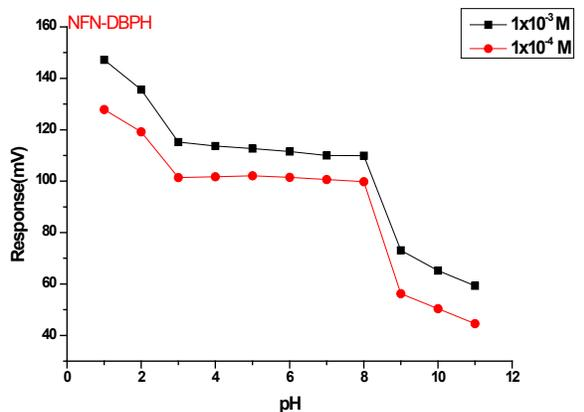
Figure 14: Effect of PH on NFN-DBPH electrode response
