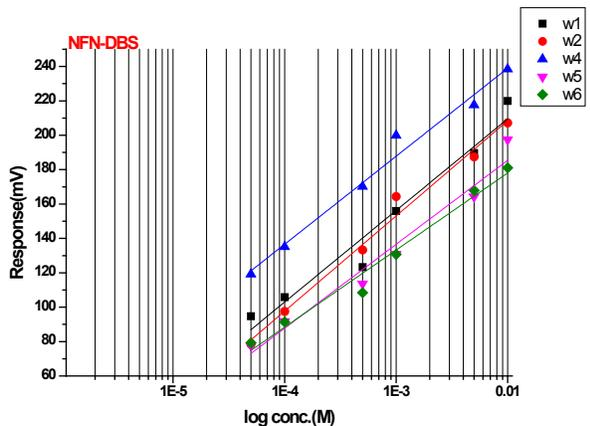
Figure 10: Life time of the (NFN-DBS) electrode.
