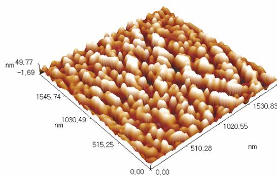
Figure 6: AFM image three dimensional of the hydrogel
