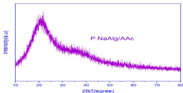
Figure 4: XRD spectrum of the hydrogel
