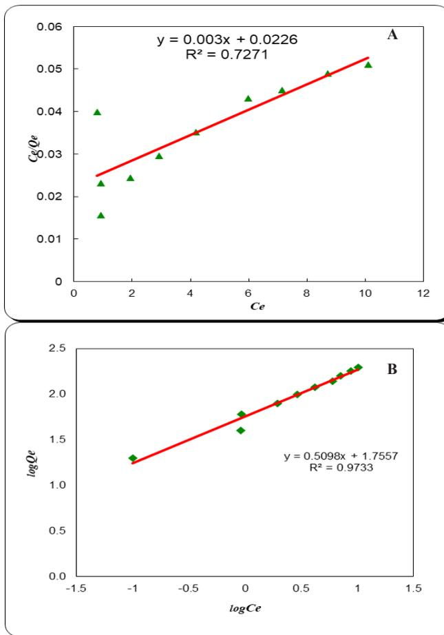
Figure 9: A: The linearized Langmuir isotherm for CV adsorption at 25°C, B: The linearized Freundlich isotherm for CV adsorption at 25 °C
