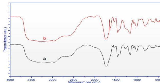
Figure 3: FTIR spectrum of (a) hydrogel (b) hydrogel after adsorption CV
