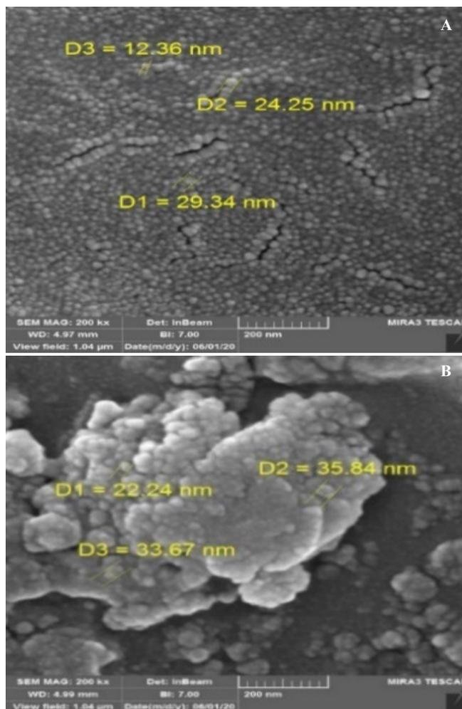
Figure 5: a: FE-SEM image of (SA-g-pAAc) hydrogel, b: after adsorption CV dye on the hydrogel
