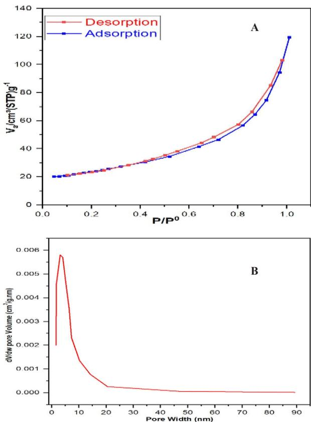
Figure 7: A: adsorbent isotherm - desorption of nitrogen N<sub>2</sub> to BET, B: adsorbent isotherm - desorption of nitrogen N<sub>2</sub> to BJH
