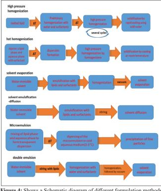
Figure 4: Shows a Schematic diagram of different formulation methods used in preparations of SLNs
