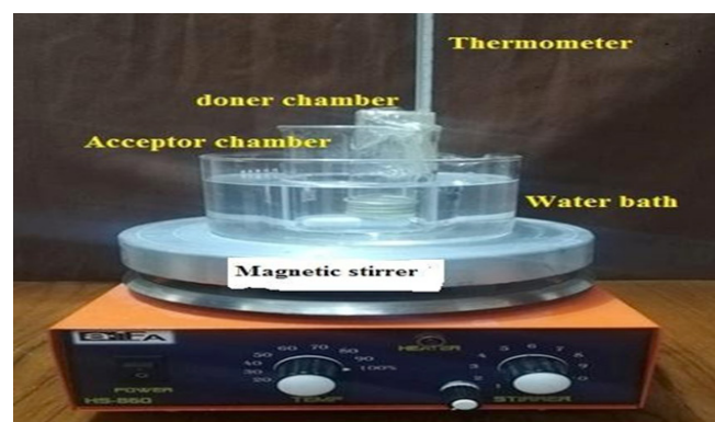
Figure 1: Modified Franz diffusion cell
