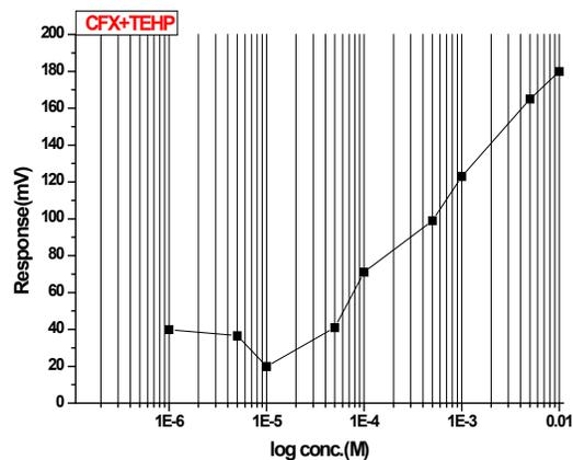
Figure 6: Calibration curve of (CFX-CV) first electrode with TEHP as plasticizer
