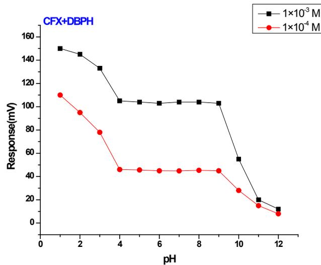
Figure 10: Effect of pH for (CFX-CV) electrode using DBPH as plasticizer
