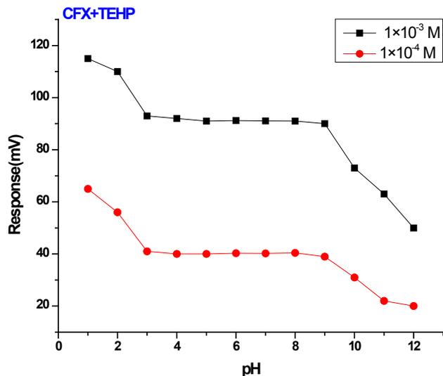
Figure 9: Effect of pH for (CFX -CV) electrode using TEHP as plasticizer
