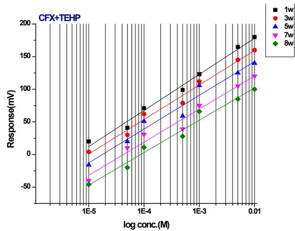
Figure 15: Life time of (CFX -CV) electrode using TEHP as plasticizer
