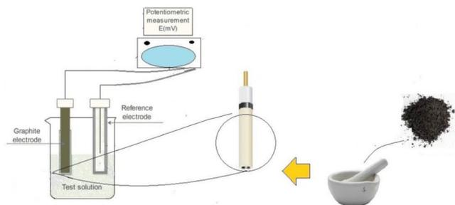
Figure 2: A diagram of the ISE cell for carbon paste electrode<sup>15</sup>
