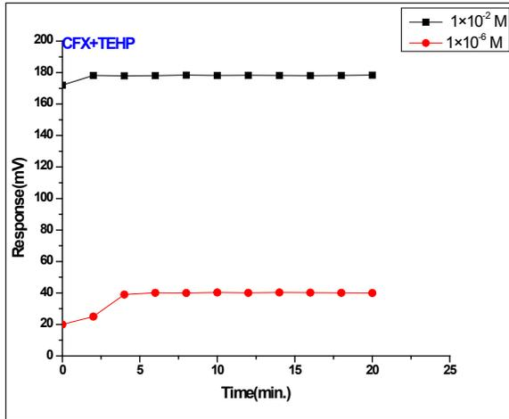
Figure 12: Response time of (CFX -CV) electrode using TEHP as plasticizer
