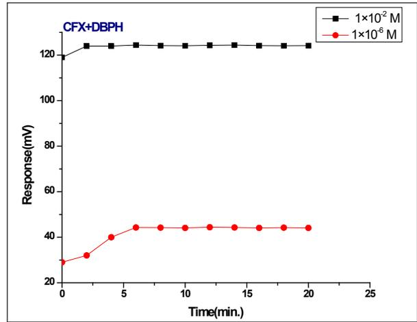
Figure 13: Response time of (CFX -CV) electrode using DBPH as plasticizer
