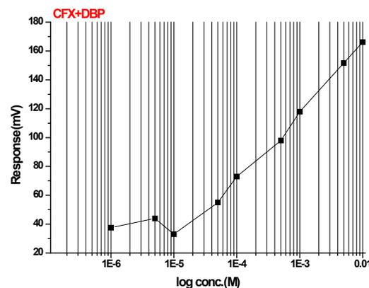
Figure 8: Calibration curve of (CFX-CV) third electrode with DBP as plasticizer
