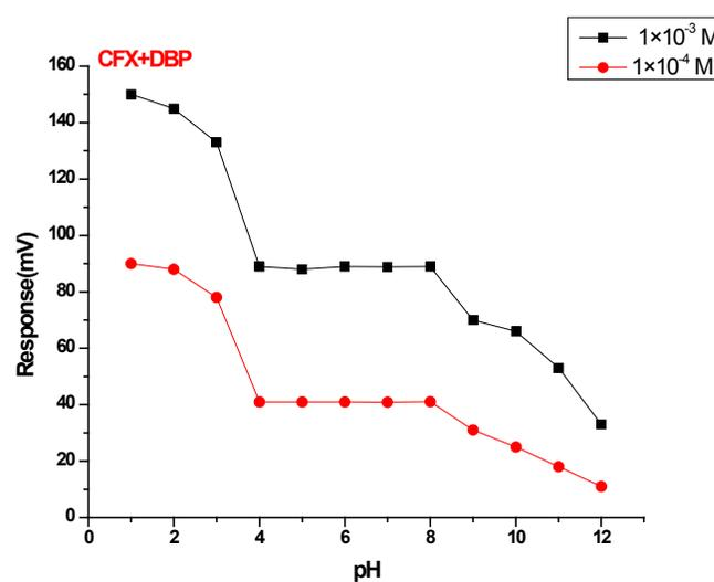
Figure 11: Effect of pH for (CFX-CV) electrode using DBP as plasticizer
