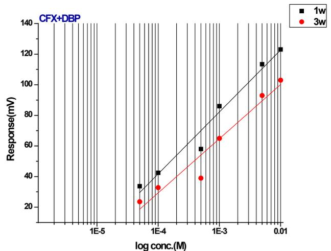
Figure 17: Life time of (CFX -CV) electrode using DBP as plasticizer
