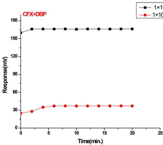
Figure 14: Response time of (CFX -CV) electrode using DBP as plasticizer
