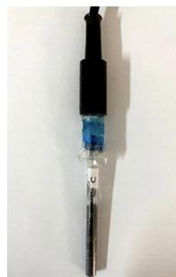
Figure 3: A carbon paste electrode
