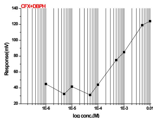
Figure 7: Calibration curve of (CFX-CV) second electrode with DBPH as plasticizer
