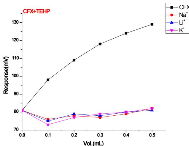
Figure 18: Selectivity for CFX-CV+TEHP for mono-cations by match potential method
