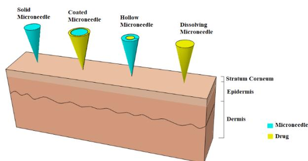
**Figure 2:** Schematic representation of various types (solid, coated, hollow, and dissolving) of microneedles.
