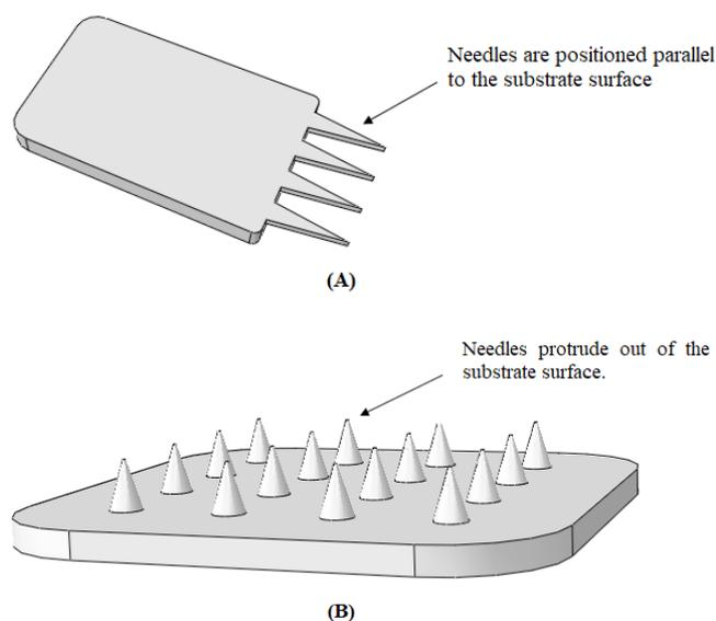
**Figure 1:** Microneedle based on the fabrication method A) In-plane microneedle and B) Out-of-plane microneedle.
