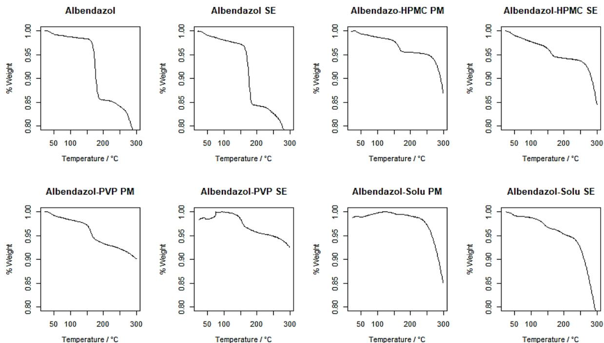
**Figure 2:** The DSC thermogram of the albendazole as received, physical mixtures of the drugs with polymers and amorphous solid dispersion of the drugs with polymers.
