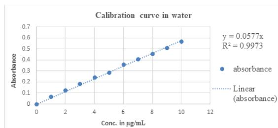
**Figure 2:** Calibration plot for lamivudine with water
