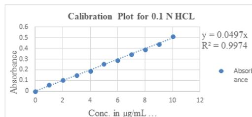
**Figure 3:** Calibration plot for Lamivudine with 0.1 N HCl
