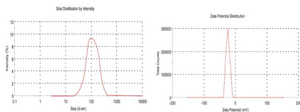
**Figure 4:** Particle size and Zetva potential of S-NPs (n=3)
