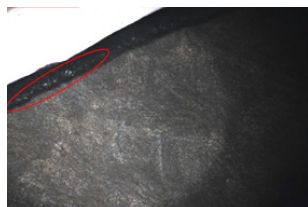
Figure 3: First sign of collapse observed as the product reaches -29°C
