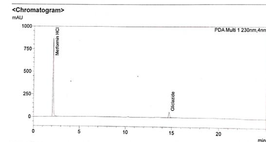
Figure 2: Chromatogram of metformin and gliclazide mix standard
