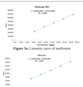
5.00 10.00 15.00 20.00 25.00 30.00 Cencentration in(ppm) Figure 3b: Linearity curve of gliclazide
