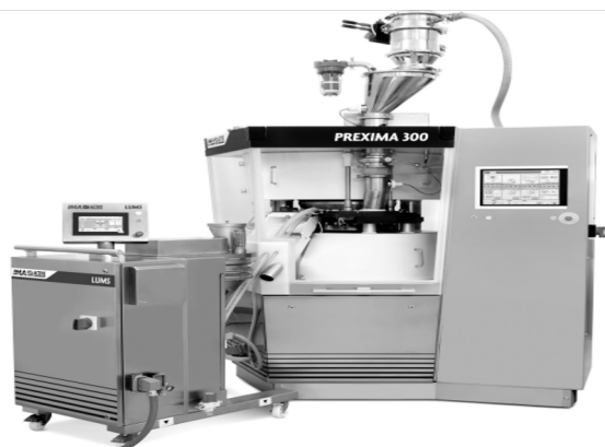
Figure 2: LUMS, dosing equipment for external lubricant addition in a tablet press (Source: From IMA S.P.A., Bologna, Italy)
