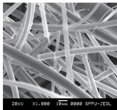
Figure 2: SEM of ITZ-Sucrose microfibers
