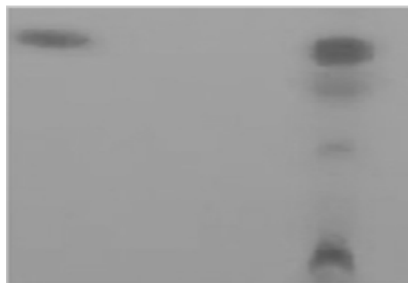
Figure 3: Thin layer chromatography for purified phenazine and the standard phenazine antibiotic
