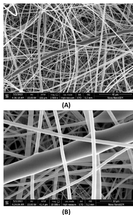
Figure 1: SEM representation of NF3 at magnification (A) 500X, (B) 2.5 KX
