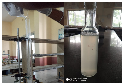
Figure 1: Extraction of allicin using glass column for the separation and purification of allicin from fresh commercial garlic samples
