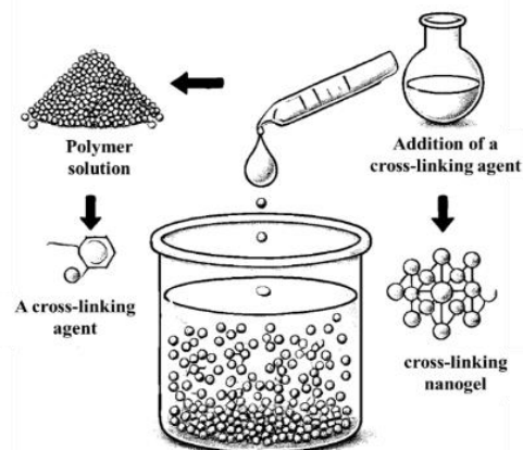
Figure 4: Formation of Cross-Linked Nanogels from a Polymer Solution using a Cross-Linking Agent.
