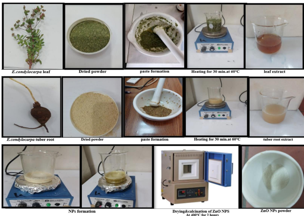
Figure 3: Preparation process of ZnO nanoparticles from leaf and tuber roots of E. condylocarpa
