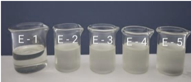
Figure 19: Pre concentrate mix consisted of Smix and sesame oil upon aqueous dispersion
