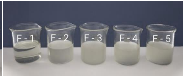
Figure 20: Pre concentrate mix consisted of Smix and oleic acid upon aqueous dispersion
