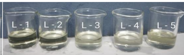
Figure 26: Preconcentrate mix consisted of Smix and oleic oil upon aqueous dispersion
