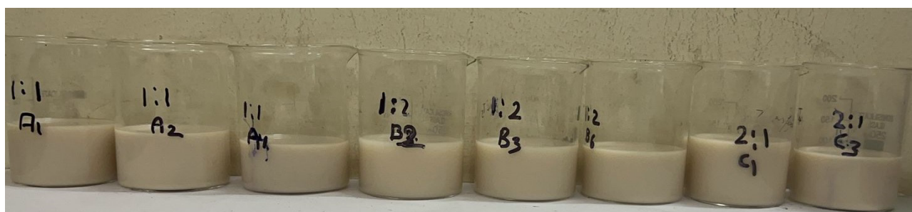
Figure 8: Representative drug-loaded nanoemulsion formulations comprising varying ratios of oil, surfactant, and co-surfactant (1:1, 1:2, and 2:1), selected based on preliminary studies for further characterization.
