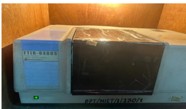
Fig 1: Shimadzu FTIR-8400S spectrophotometer used for infrared spectral analysis
