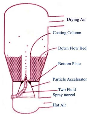
**Fig. 6: Fluidized Bed / Spray Coating technique<sup>19</sup>**
