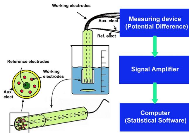
**Fig. 7: Evaluation of taste using e-tongue<sup>55</sup>**
