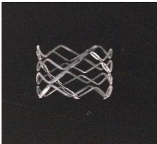
Fig. 1: The bioabsorbable stent made of PLLA.
