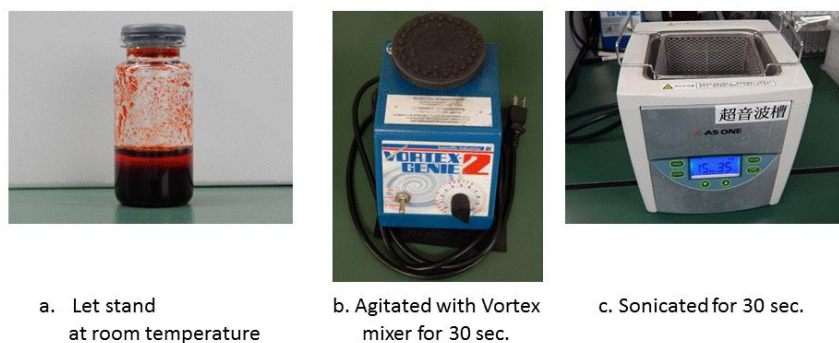
Figure 1: Loading procedures of epirubicin into DC Bead. Mixtures of epirubicin solution and DC Bead were (a) let stand at room temperature, (b) agitated for 30 seconds with Vortex mixer, and (c) sonicated for 30 seconds with ultrasonic cleaner.
