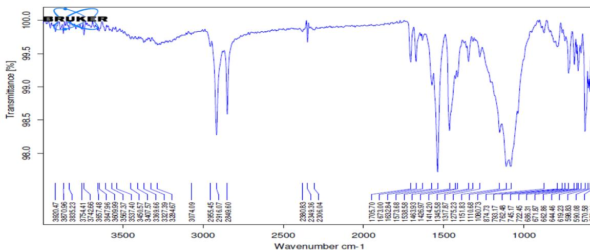
Figure 4: FT-IR Spectrum of Optimized formulation.
