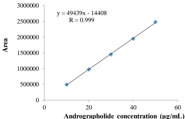
Figure 3: Andrographolide calibration curve in HCl pH 3.4.
