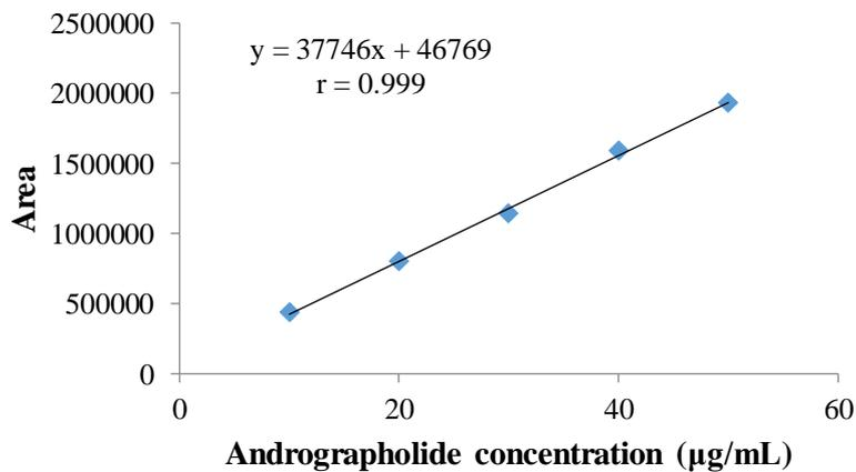
Figure 2: Andrographolide calibration curve in phosphate buffer pH 6.8.
