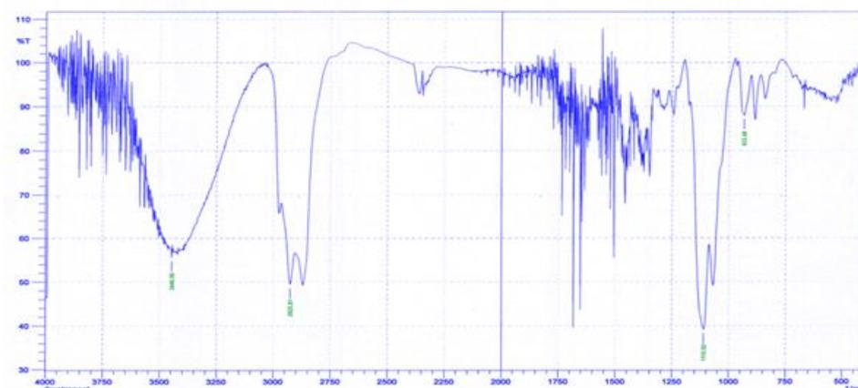
Figure 3: FTIR spectra obtained for optimized formulation IBU29
