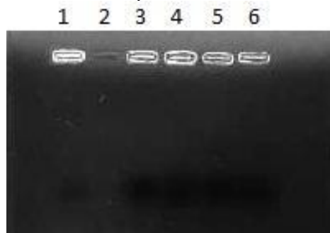
Figure 3: Agarose Gel Electrophoresis 0.8% agarose gel analysis of DLCNP (Well 1, 3, 4, 5 and 6 prepared at 0, 6,12, 18, 24 th day respectively) and Supernatant (after the formation and before the washings of DLCNP) (Well 2).
