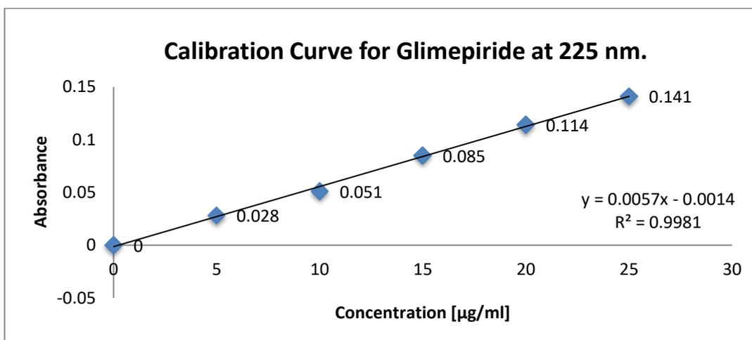
Figure 2: Standard Calibration Curve for Glimepiride at 225 nm.
