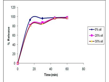
Fig. 3: Comparative dissolution profile of paracetamol at 75 rpm using different percentage of oil in dissolution media
