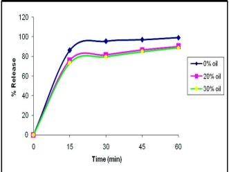
Fig. 2: Comparative dissolution profile of nimesulide at 75 rpm using different percentage of oil in dissolution media
