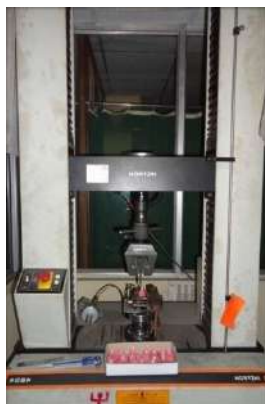
Figure 13: Loading of the sample for shear bond testing
