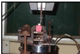
Figure 12: Shear bond testing
