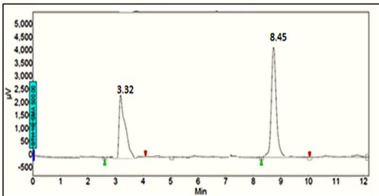
**Figure 5: Chromatogram of hydrogen peroxide-induced degradation**
