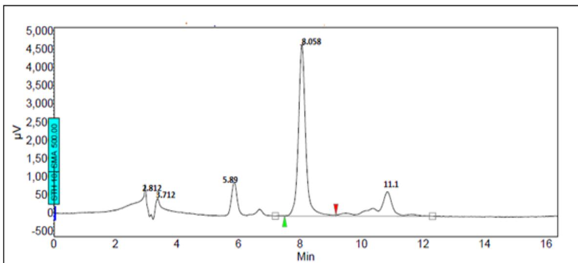
Figure 1: Standard chromatogram of retinol acetate by RP-HPLC
