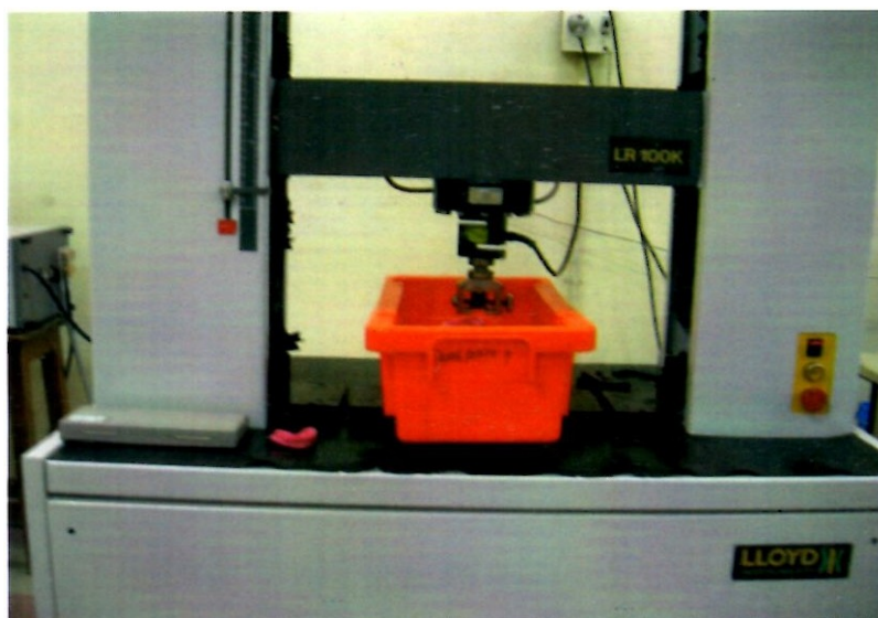
Figure 4: Instron testing apparatus illustrated with water bath maintained at 37°C
