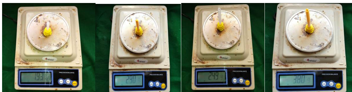
Fig 3-6: Before and after weights of Yellow T- mixer and Conventional helical mixing tips.
