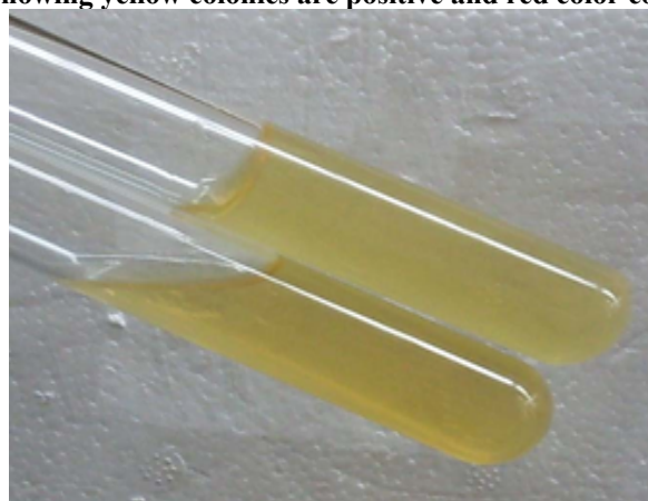
Gelatine liquefaction test showing gelatine liquefaction negative(top) and gelatine liquefaction positive (bottom)
