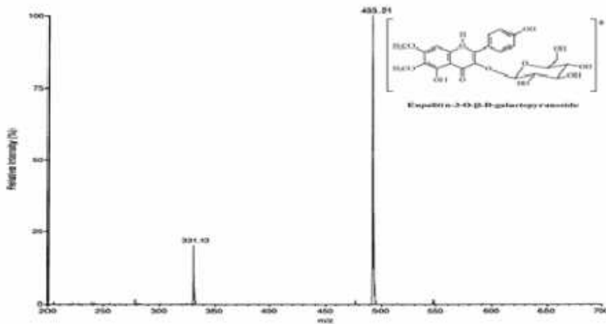
Figure 2: Mass spectrum of Eupalitin-3-O-β-D-galactopyranoside in positive ion mode
