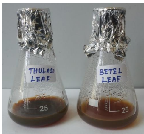
Figure 1: Silver nano particles prepared by the plant extracts
