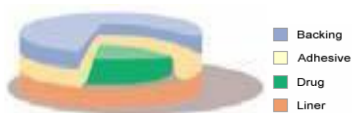
Figure 8: Single layer drug in adhesive patch with its different Component.
